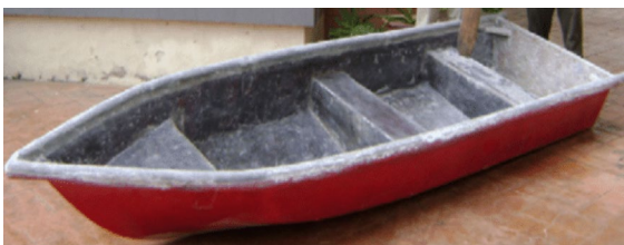
Fig. 2 Sugar palm biocomposite boat (Ishak et al. 2013). Reproduced with permission from Ishak et al. 2013. Copyright 2013 Elsevier
