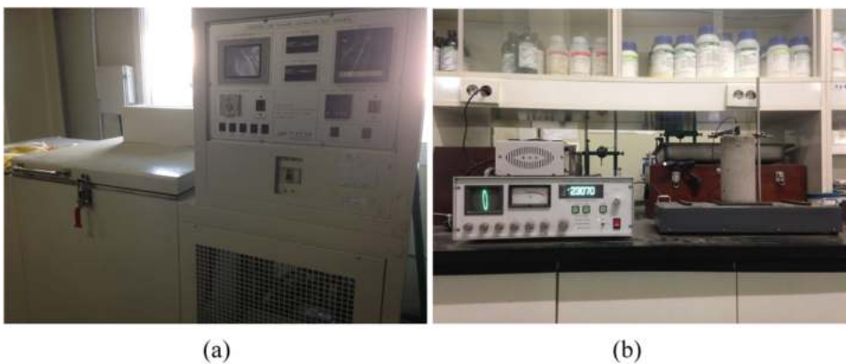
Fig. 12. (a) Freeze-thaw test machine; (b) dynamic elastic modulus measuring equipment.
