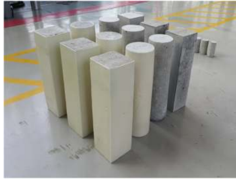
Fig. 14. Photo of uniaxial compression test RC specimens with (white) and without STPU strengthening (gray).
