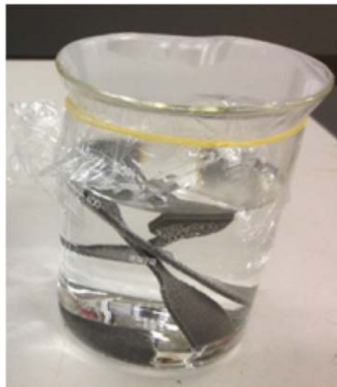
Fig. 8. Acid environmental exposure test under acid concentration of \text{H}_2\text{SO}_4 2 % 400 mL.
