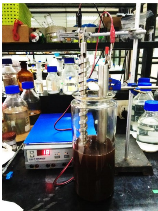
Figure S2. Cathodic reduction and electrophoretic deposition setup.
