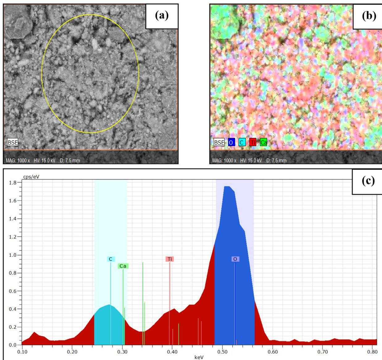
Fig. 4. (a) SEM images, (b) EDX mapping, and (c) percentage element of TiO<sub>2</sub>/eggshell (3:7).
