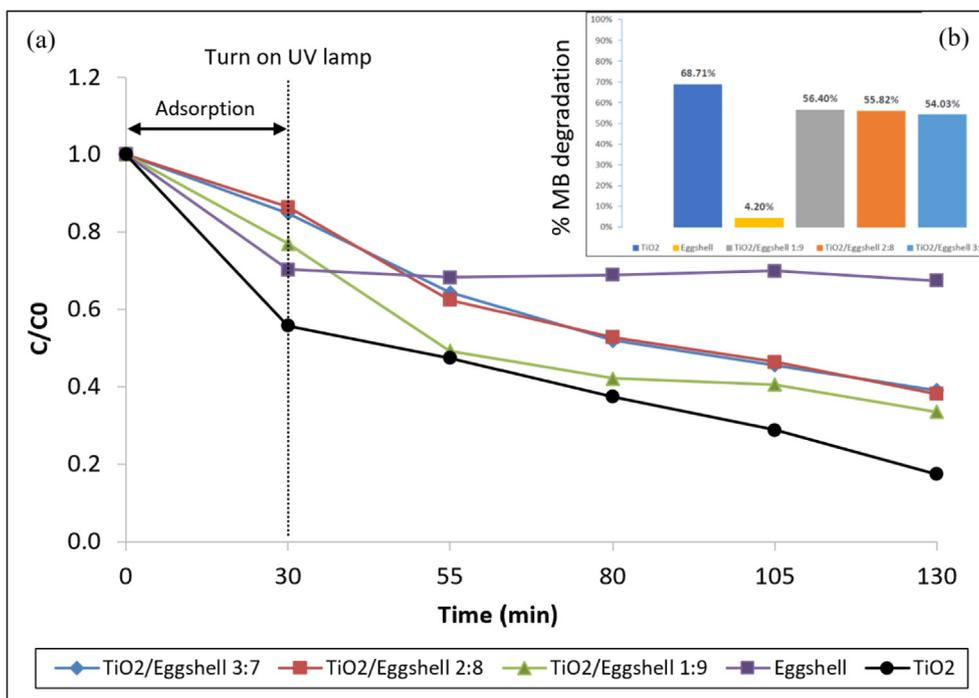
Fig. 6. (a) Normalized degradation behavior of MB using different types of photocatalyst and (b) MB percentage degradation.
