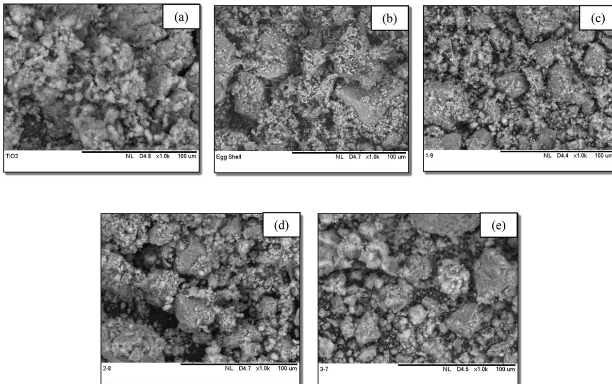
Fig. 3. SEM images of (a) TiO<sub>2</sub>, (b) eggshells, (c) TiO<sub>2</sub>/eggshell (1:9), (d) TiO<sub>2</sub>/eggshell (2:8), and (e) TiO<sub>2</sub>/eggshell (3:7) with 5 k of magnification.
