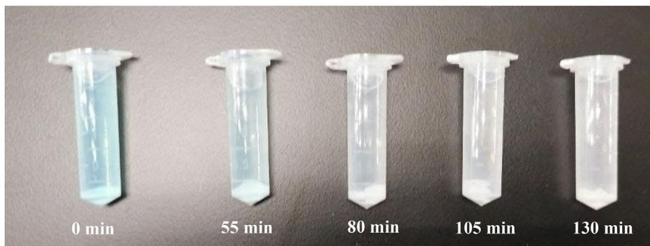
Fig. 5. Reduction color intensity of MB during photocatalytic experiment.
