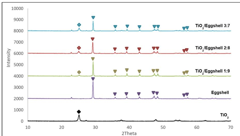
Fig. 2. XRD patterns of eggshells, TiO<sub>2</sub>, TiO<sub>2</sub>/eggshell (1:9), TiO<sub>2</sub>/eggshell (2:8), and TiO<sub>2</sub>/eggshell (3:7).
