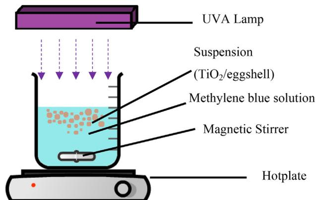
Fig. 1. Schematic diagram of the suspension system for MB photocatalytic activity testing.
