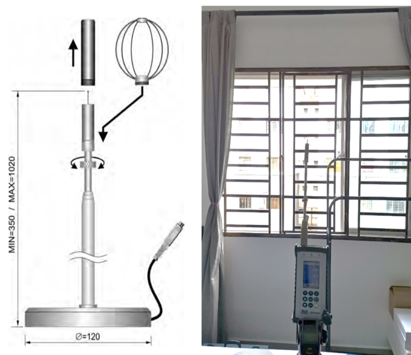
Figure 5. AP471S wind velocity hotwire airspeed probes [14] (left), and setup of field measurements (right).
