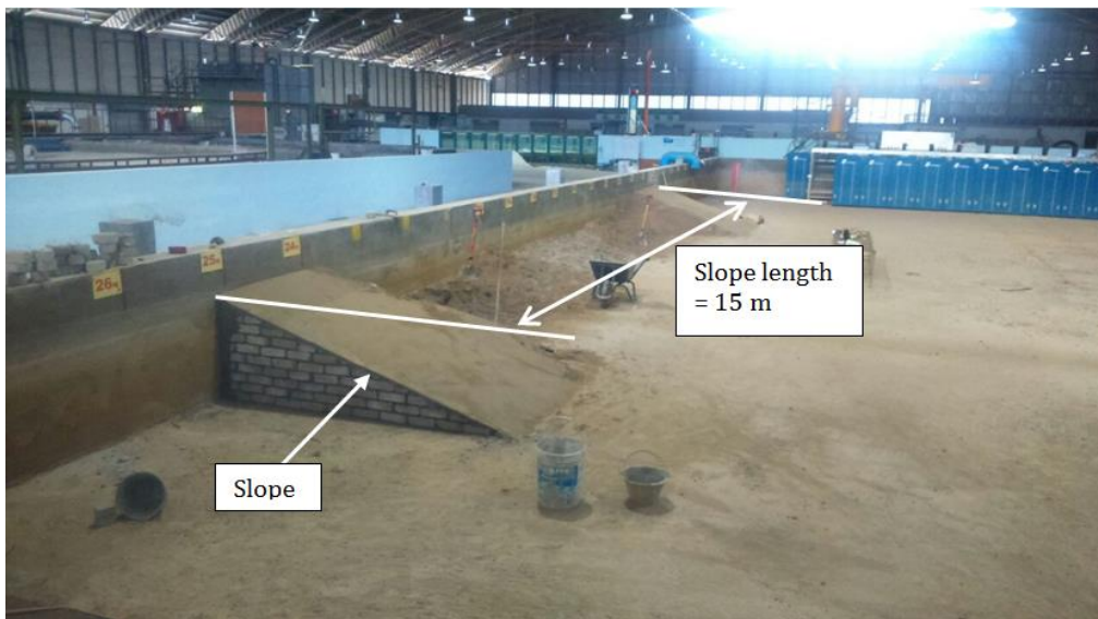
Fig. 10 Slope setup under preparation at NAHRIM facility for model testing
