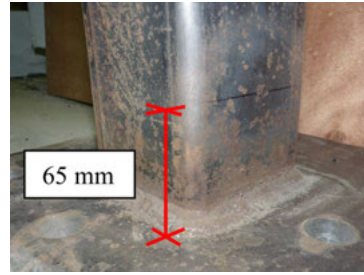
(b) Deformation of NCFHS-0 (right face)
