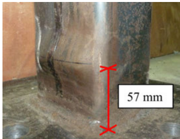
(c) Deformation of NCFHS-20 (left face)
