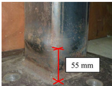
(c) Deformation of RuPCHS-20 (left face)
