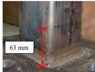
(b) Deformation of RuPCHS-0 (right face)
