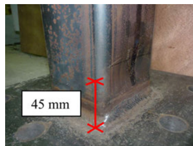
(d) Deformation of SHS-20 (right face)
