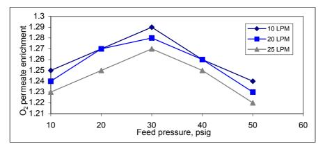
Figure 3 O<sub>2</sub> permeate enrichment versus feed pressure
