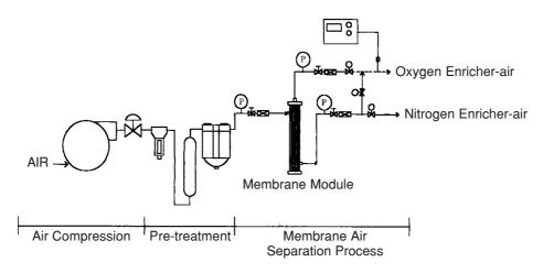
Figure 1 Schematic system flow diagram
