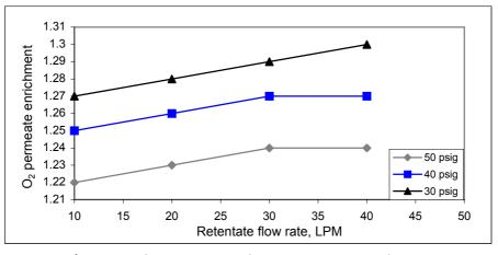
**Figure 4**  $O_2$  permeate enrichment versus retentate flow rate
