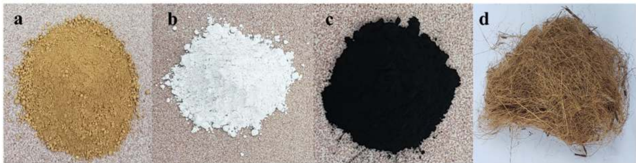
Figure 2. Image of (a) soil, (b) lime, (c) activated carbon, (d) coir fibre.
