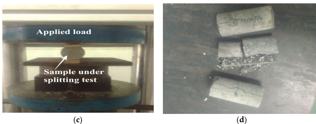
Figure 3. Testing of concrete cylinders: (a) cylinder under compressive test; (b) cylinders after compression tests; (c) cylinder under splitting test; (d) cylinders after splitting tests.
