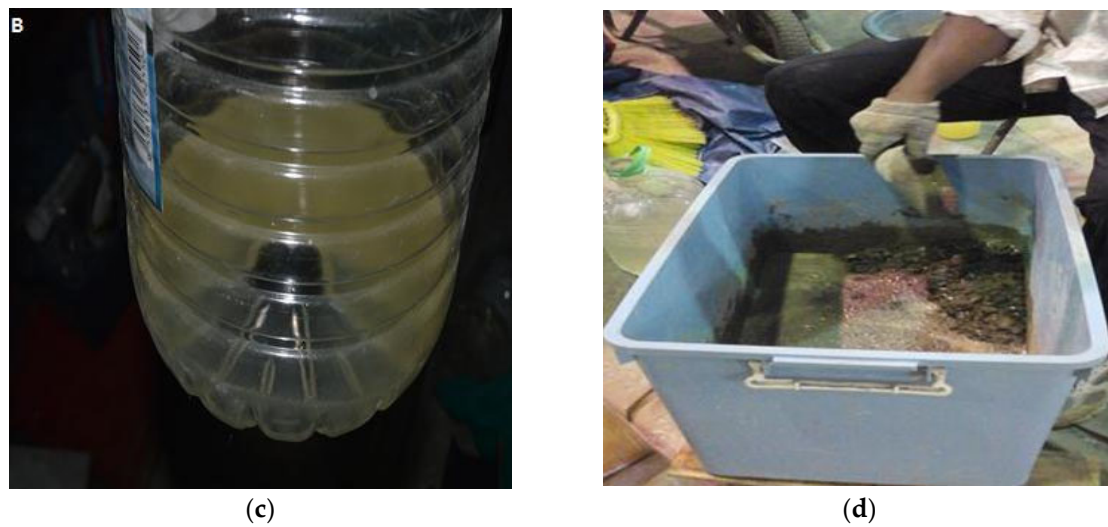
Figure 2. Illustrations of the concrete materials: (a) fine aggregate in the oven; (b) coarse aggregate; (c) Glenium ACE 388; (d) mixing process.
