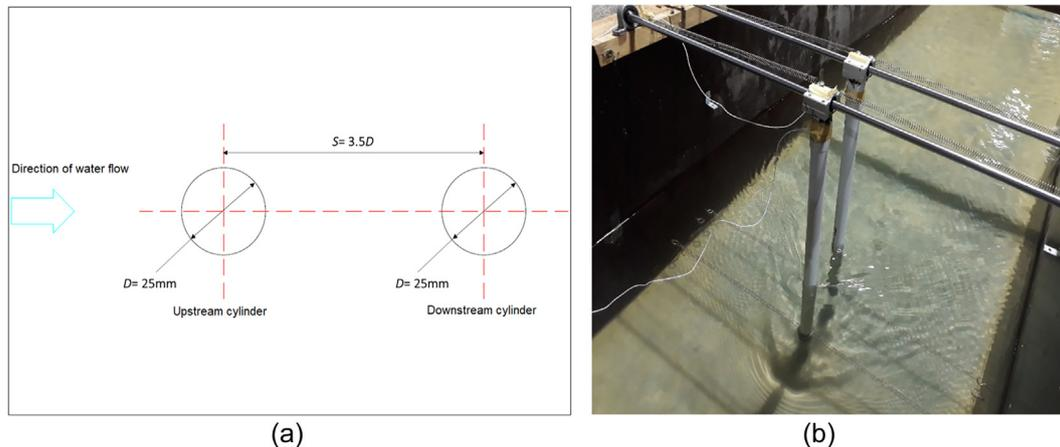
Fig. 2. (a) Schematic diagram of the cylinder arrangement; (b) the experimental set up of the cylinder in the tandem.
