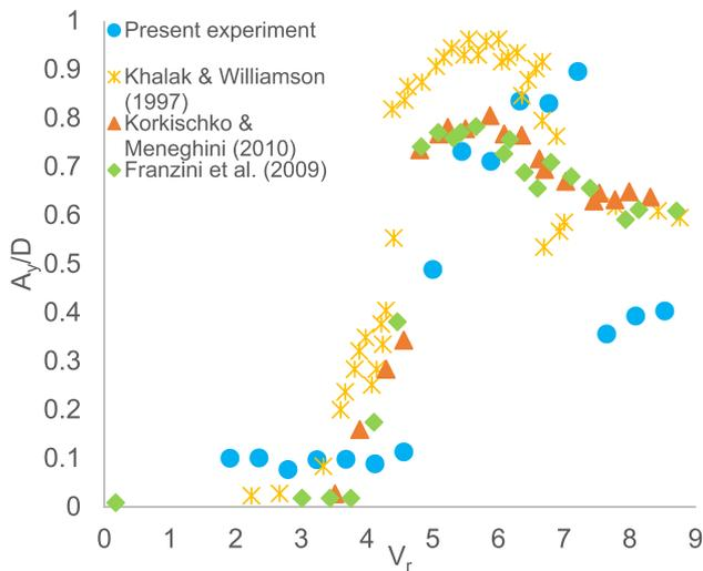
**Fig. 4.** Amplitude response of a single circular cylinder versus reduced velocity.
