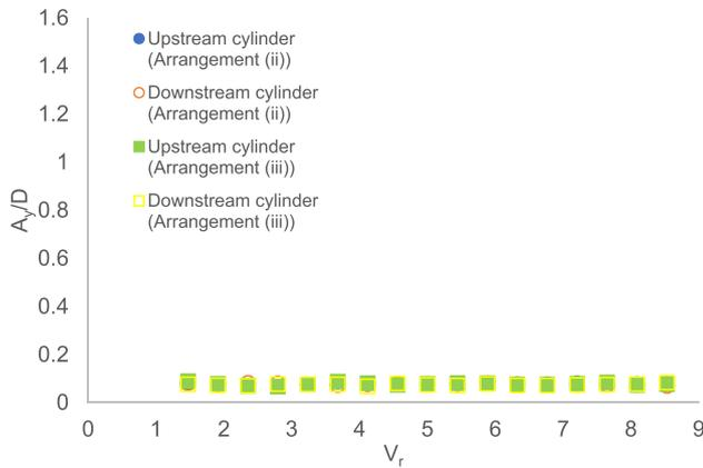
Fig. 10. Displacement response of the upstream and downstream cylinder versus reduced velocity (Arrangements (ii) and (iii)).
