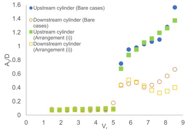
Fig. 9. Displacement response of the upstream bare and downstream straked cylinder versus reduced velocity (Arrangement (i)).
