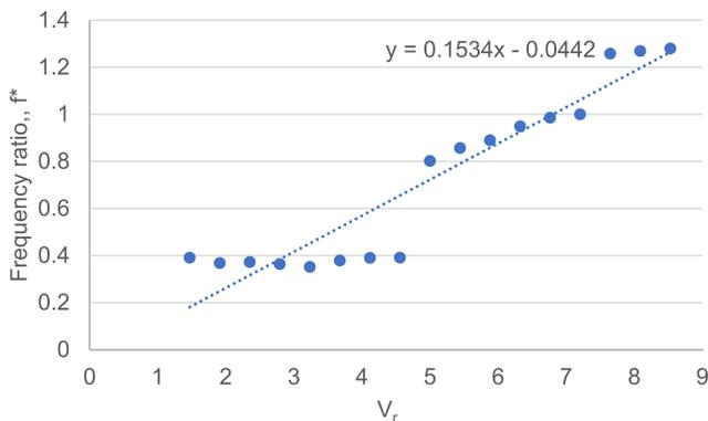
**Fig. 5.** Frequency response of a single circular cylinder versus reduced velocity.
