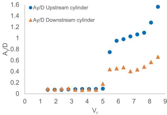
Fig. 7. Amplitude response of upstream and downstream cylinders without helical strake versus reduced velocity.
