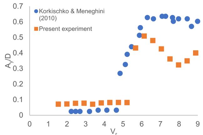
Fig. 12. The comparison of displacement response of downstream with helical strake cylinder versus reduced velocity at Arrangement (i).
