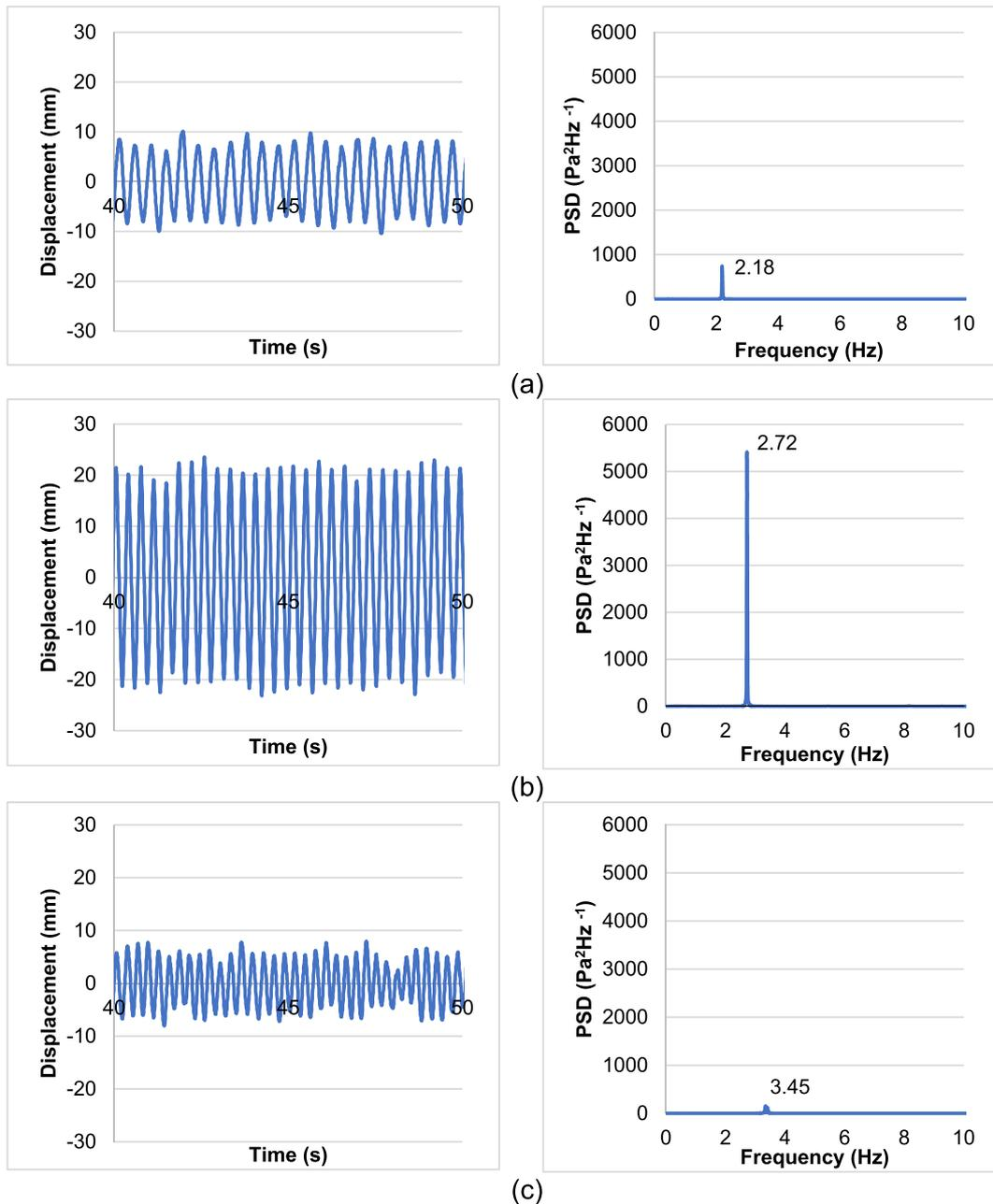
Fig. 6. The time series of displacement and frequency spectra of cross-flow vibrations of single circular cylinder at reduced velocity of (a) 5.0, (b) 7.2 and (c) 7.6.
