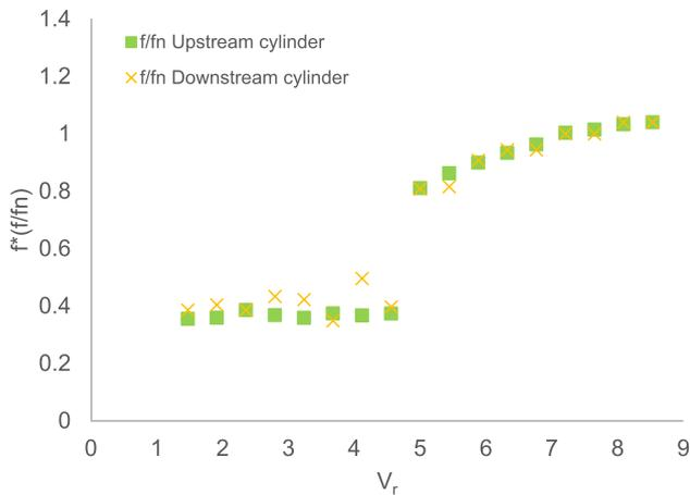
Fig. 8. Frequency response of upstream and downstream cylinders without helical strake versus reduced velocity.
