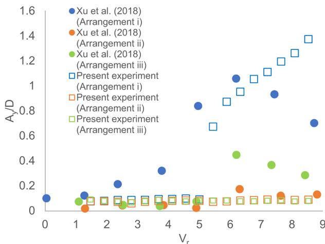
Fig. 11. The comparison of displacement response of upstream without and with helical strake cylinder versus reduced velocity at all arrangements.
