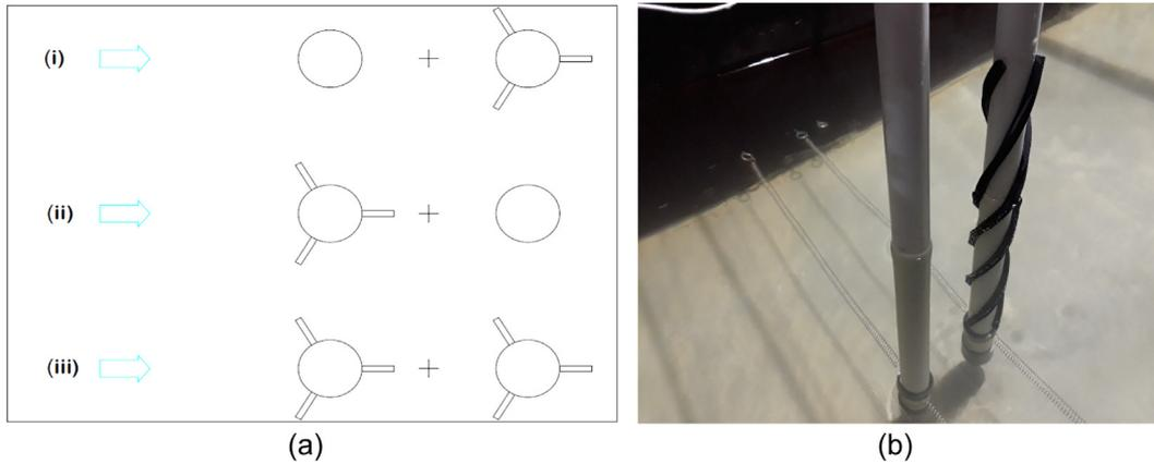
**Fig. 3.** (a) Helical arrangement of two tandem cylinders: (i) Upstream (Bare) and Downstream cylinder (with helical strake); (ii) Upstream (with helical strake) and Downstream cylinder (Bare); and (iii) Upstream (with helical strake) and Downstream cylinder (with helical strake), (b) Example of helical strake installation for Arrangement (i).
