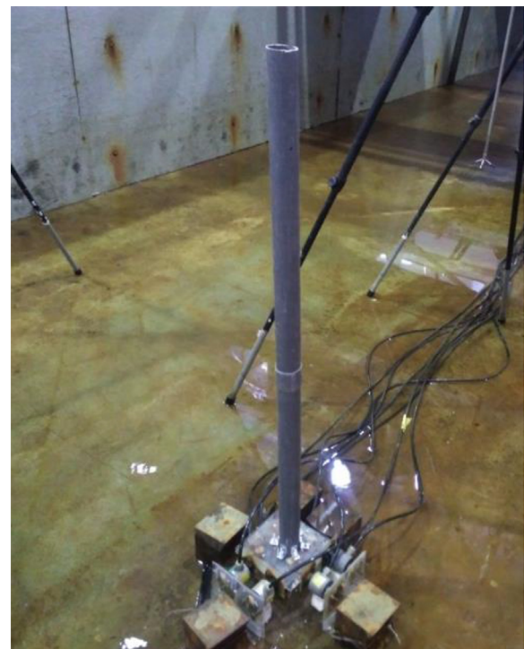
Fig. 2. Vertical circular cylindrical model with the 3D force transducer.
