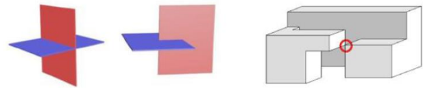
(a) Self-intersections (b) Non-manifold vertex Figure 2. Some limitations of the detect and local repair method (Alam et al., 2014).
