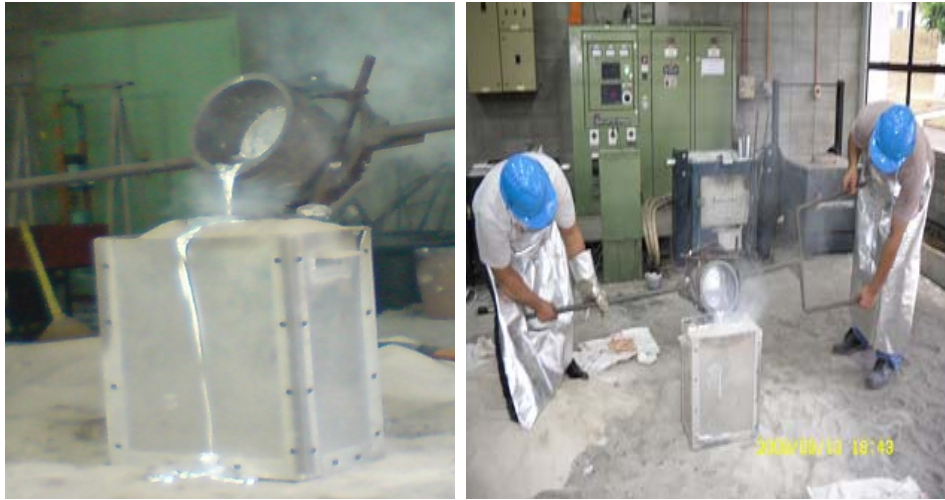
Figure 3.10: Pouring of castings
