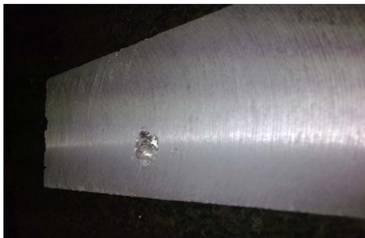
Figure 4.13: Some of the defects observed in the castings (gas porosity, penetrate of coating into the metal and shrinkage)
