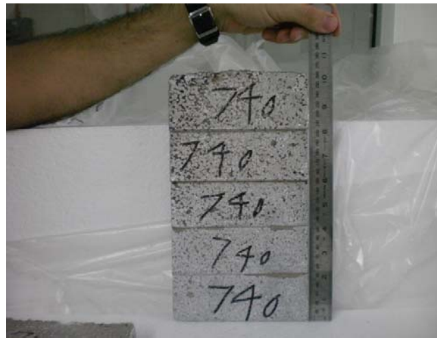
Figure 4.1: Castings using 16, 20 and 32 foam density
