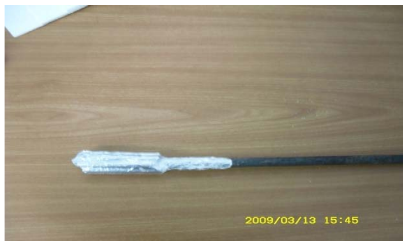
Figure 3.8: Shaft used to mixed the TiB
