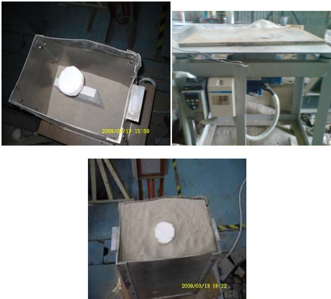
Figure 3.7: sand filling and vibration
