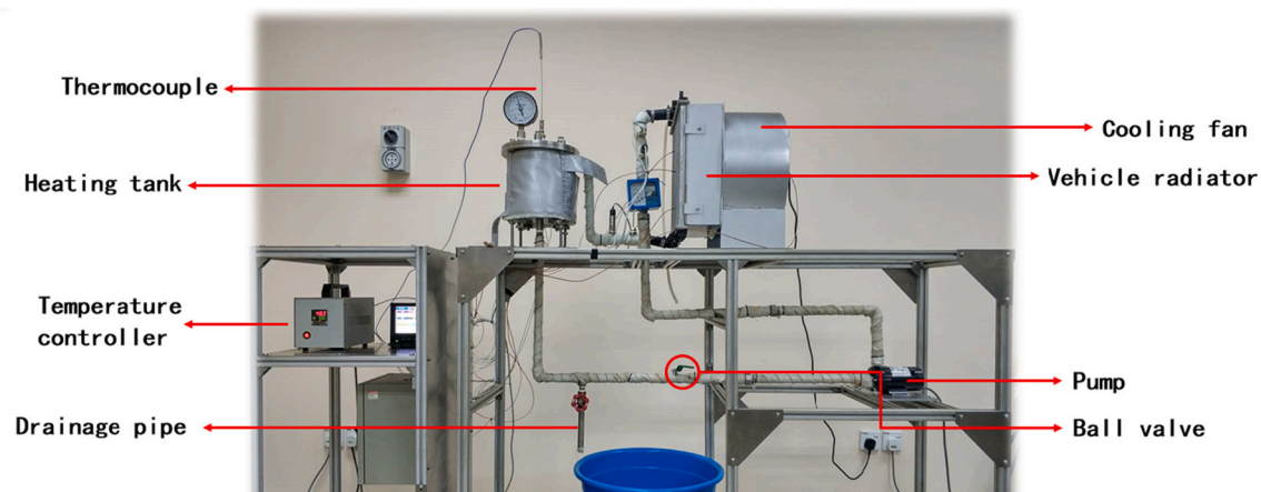
Fig. 1. Test rig for obtaining heat transfer performance of the coolant.
