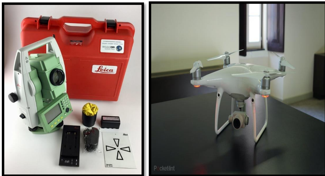
Figure 1. 1 Leica TS06+ (Reflectorless) and DJI Phantom 4 Pro (UAV)
