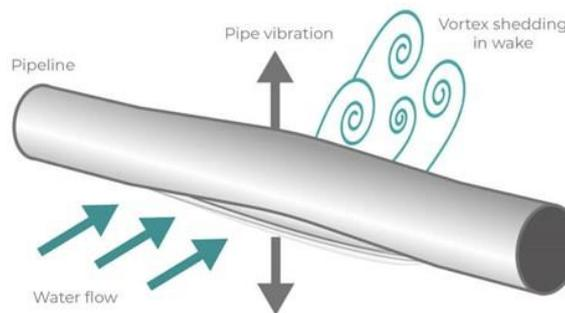
Figure 1.2 The formation of vortex shedding behind a pipeline, reproduced from ATMOS International (2022)
