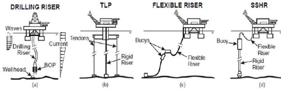
Figure 1.1 Types of riser system configurations used in oil and gas production, namely (a) free-standing riser, (b) top-tensioned risers (TTRs), (c) catenary riser (lazy-wave), and (d) hybrid riser tower, reproduced from Murai & Yamamoto (2010)
