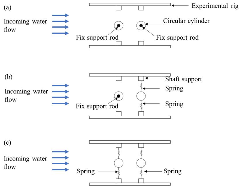
Figure 1.4 Definition sketch of different cylinder's set-up in tandem configuration. (a) fix- fix, (b) fix- vibrate, and (c) vibrate-vibrate cylinder
