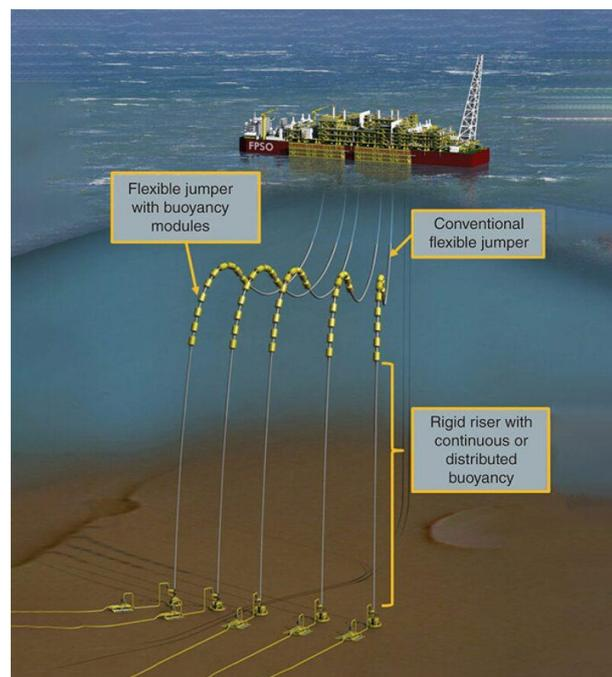
Figure 1.3 The hybrid riser tower with more than one rigid riser, reproduced from Carpenter (2020)
