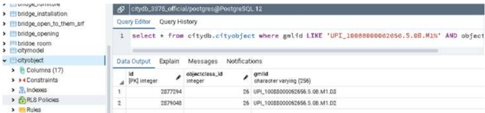
Fig. 25. A building of UPI_10088000062656.S.0B.M1 has two representation LoD2 (...D2) and LoD3 (...D3) as shown in the output query
