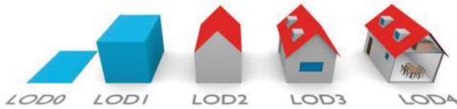
Fig. 1. Five LoDs introduced in CityGML 2.0
