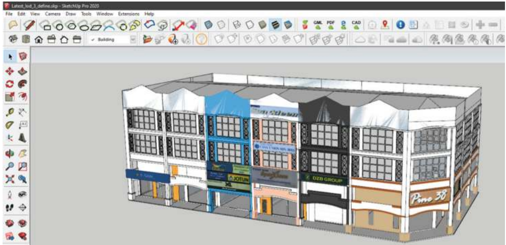
Fig. 30. Example of LoD3, with the texture of a building block separated by building ownership (each lot) as a final result at SketchUp software
