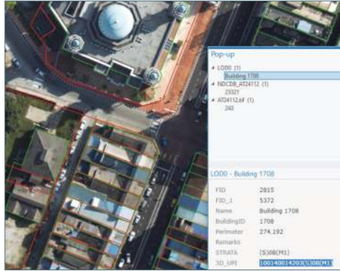
Fig. 11. Example of LoD0 (building footprint, light green vector) in relation to the 2D lot (colored red)
